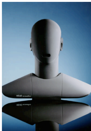
Figure 4.27. The AACHEN Head Model HMS II, manufactured by HEAD acoustics. The outer ears are designed according to a "structural averaging" of HRTFs; note the inclusion of the upper torso. Two versions of the head are available: the HMS II, intended for analysis within an integrated system, and the HRS II, for recording studio applications. Photograph courtesy of Wade Bray, Sonic Perceptions-HEAD acoustics.
